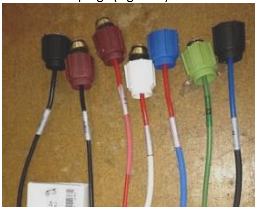
Figure 2. ‘Fuse Cap’ terminated lead example.
